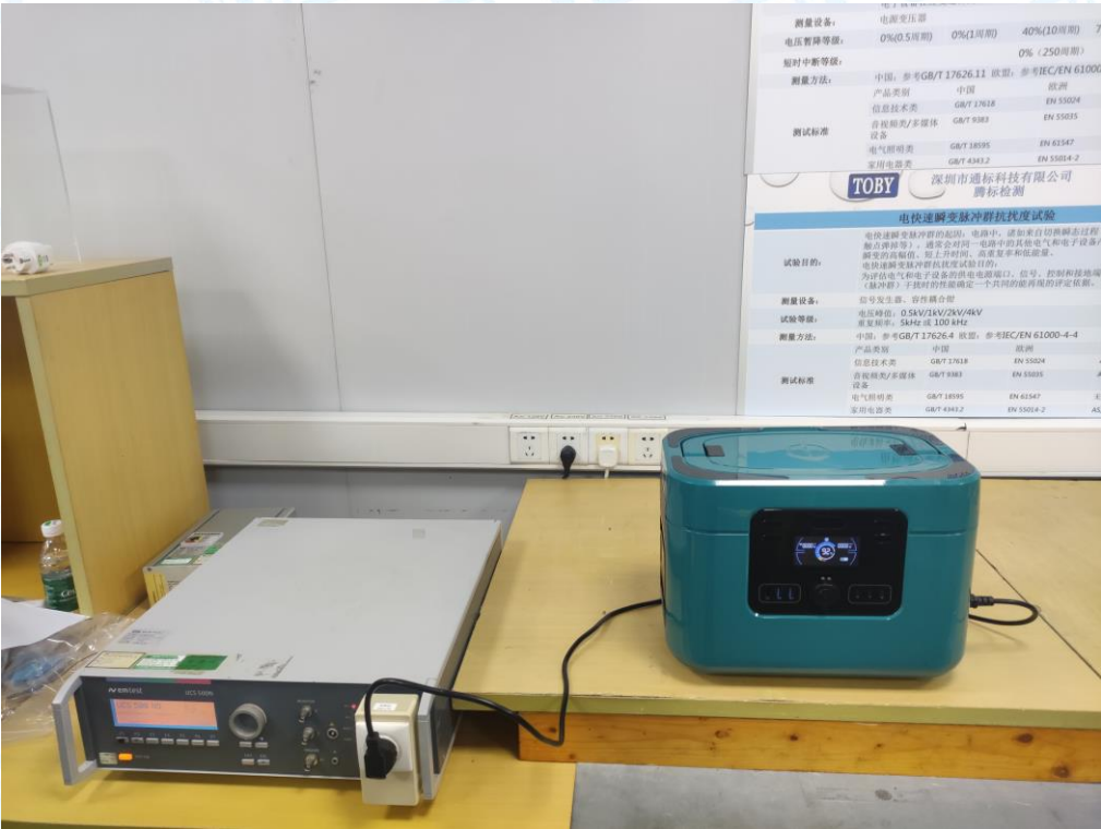
Radio-frequency, Continuous Conducted Disturbance Test Setup
